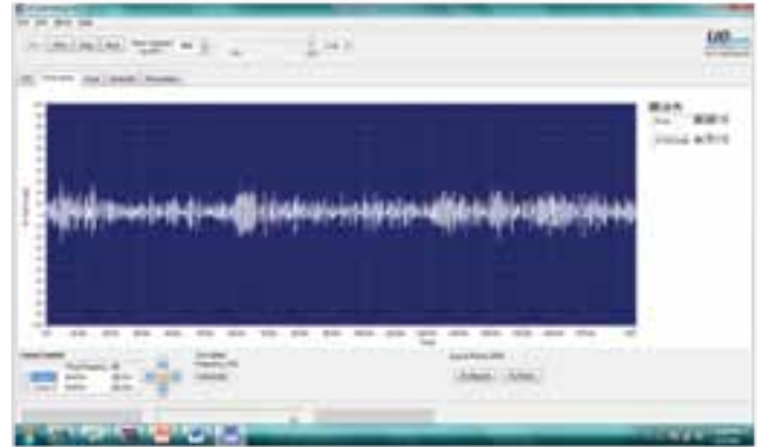
Figure 4b: Energy-based time plot for a properly lubricated bearing (Image courtesy of UE Systems, Inc.)
