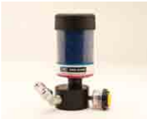
Figure 1: This fitting can be used to replace a standard fill port on a hydraulic or lube oil reservoir to allow for the non-intrusive addition of make-up oil. The breather port on top is fitted with a desiccant breather capable of excluding both particles and moisture.
