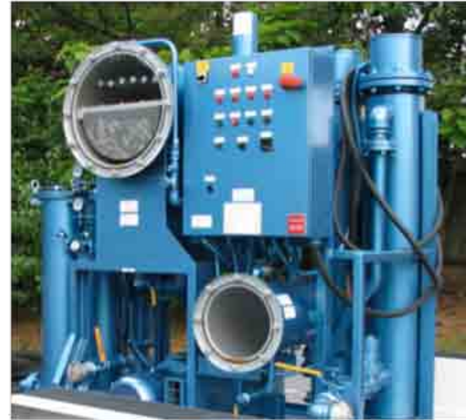
Figure 3: Example of a skid mounted vacuum dehydrator
