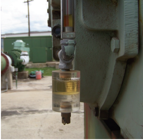
Figure 3: Installed at the lowest point on a wet sump, a BS&W bowl is an excellent way to observe free or emulsified water in oil
