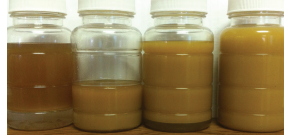
Figure 5: Simple field demulsibility tests can be very insightful in diagnosing the source of clarity problems within an oil sample
